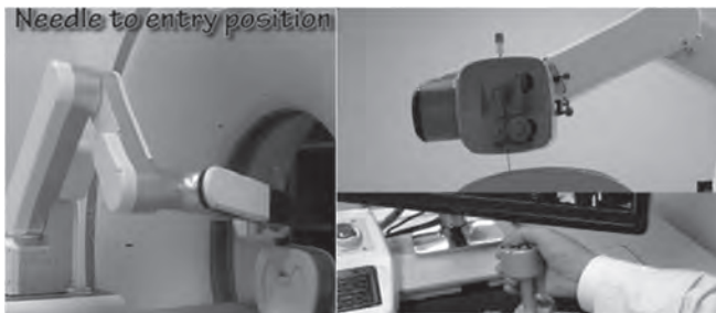
Fig. 1 CT fluoroscopy guided needle placement robot for biopsy and radiofrequency ablation made by Asan Medical Center and Hyundai Heavy Industries Co., Ltd.
